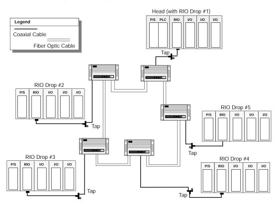
The RIO signal is sent down both legs of the ring by the drop repeater simultaneously to the head repeaters. A feature is built into the repeaters so that when a signal is received on one of the Rx lines the other Rx channel is blanked—this prevents the same signal from being transmitted twice in the ring.
