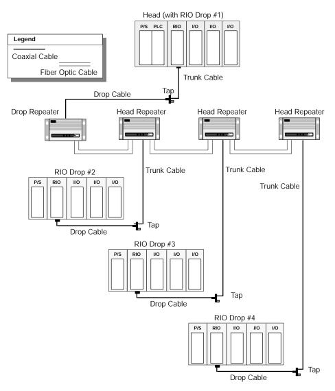
The number of chained repeaters that can be linked in a bus topology like this is determined by the total pulse width distortion (jitter) that occurs on the system (see Section 2.15 on page 46 for the calculation).
