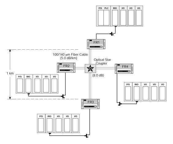
The specified power loss budget for a link using this optical cable is 16.5 dB. The cable attenuation over 1 km is 5 dB, and an attenuation of 8 dB is specified for the star coupler device itself. Two ST connectors for the Tx and Rx lines through the star coupler incur 1 dB loss each. Thus, we have a total optical power loss of:
