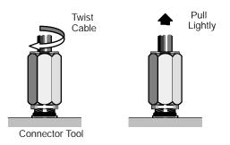
**Step 7** Disconnect the F connector from the installation tool.
