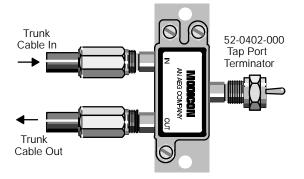
Step 3 Connect the F connector on the drop cable to the drop-cable tap port.
