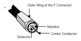
**Step 4** Tighten the F connector nut onto the 60-0528-000 RG-6 Installation Tool connector with a  $^{7}$ /<sub>16</sub> in torque wrench to 47 ... 57 in/lb of torque. Then pull on the cable to test the integrity of the connection. If the cable pulls out of the connector, begin the procedure again.
