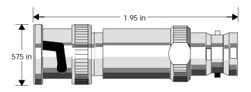
The 60-0513-000 In-line Terminator has two BNC connectors—a female for the incoming drop cable and a male to connect to the drop adapter. It has a return loss of 20 dB (VSWR 1.2:1), a frequency range from DC ... 300 MHz, and an insertion loss of 0.03 dB.
