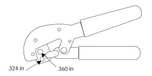
The Modicon 043509432 Crimp Tool is used to install BNC connectors onto RG-6 cable. The tool makes two sizes of hex crimp: 0.276 and 0.325 in.
