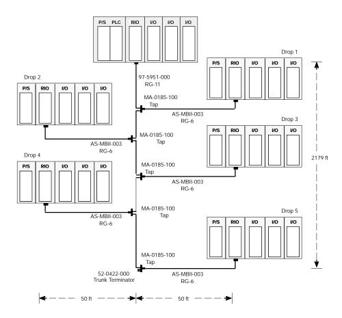
This system uses (Modicon 97-5951-000) RG-11 cable for the trunk; its specified attenuation is 0.24 dB/100 ft at 1.544 MHz. Running to the adapter at drop 5 is a Modicon AS-MBII-003 RG-6 drop cable, a 50 ft cable with an attenuation of 0.3 dB. To calculate end-to-end attenuation on the trunk cable (*TCA*), multiply 0.24 dB (the trunk attenuation per 100 ft) by 21.79:
