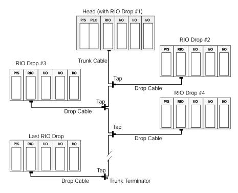
Note Because this example uses local I/O at the head, the first remote drop in the network will be I/O mapped as drop #2. If the PLC you are using does not support local I/O—e.g., the 984A/B PLCs—then the first drop in the I/O network will be I/O mapped as drop #1.
