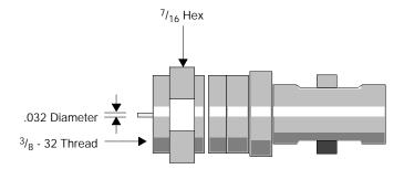
All terminators used on the RIO network must have a power handling capability of at least  $^{1}/_{4}$  W. Terminators designed for power-handling, CATV applications, or broadband cable applications cannot be used on an RIO network—they do not work in the RIO frequency range and will cause signal distortion.
