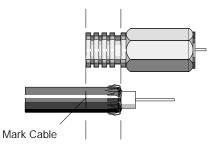
**Step 2** Using a twisting motion, push the cable firmly into the end of the F connector in the MA-0329-001 Cassette until the cable mark lines up with the end of the crimp ring.
