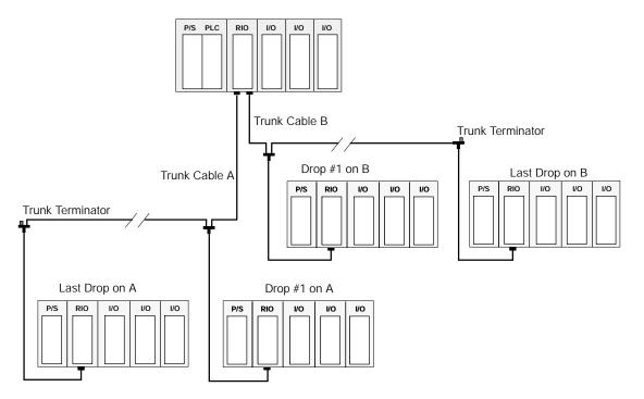
The lengths of the trunk cables and the number of drops from each do not need to be balanced in a dual cable system. In most respects, the two lines can be installed as if they were two independent cable systems, with two special considerations:
