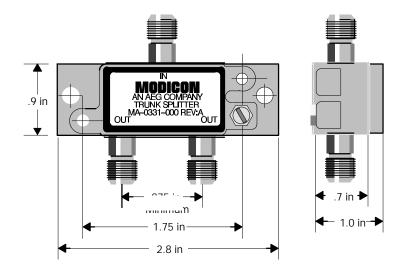
MA-0186-100 splitters have a minimum return loss of 18 dB on each port. Any unused port must be terminated. The splitter is installed between two PLCs in the main trunk cable and has three connectors (ports) on it. Each port is attenuated 6 dB from the other ports. All ports are split equally.
