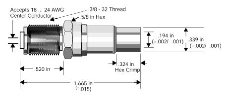
Both of these self-terminating F adapters have a return loss of 22 dB, a frequency range from 100 kHz ... 30 MHz, and an insertion loss of 0.03 dB.
