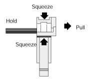
Step 4 Open the jaws and remove the cable. The dielectric plug and <sup>1</sup>/<sub>8</sub> in of the outer cable jacket should be cut from the cable. Remove any long braid strands remaining around the prepared cable end. (Long braid strands may indicate that a new blade pack is needed.) Remove any dielectric on the exposed center conductor.
