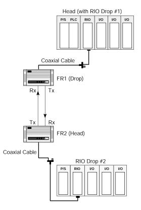
Here is a typical point-to-point RIO fiber optic link:
