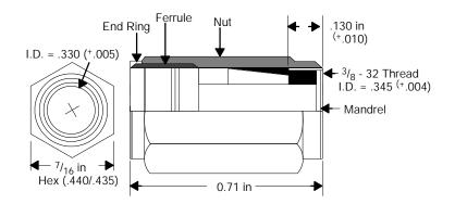
This industrial grade connector has an environmental seal on the back end and uses a boot over the female port to environmentally seal the front of the connector. It does not have a center pin connection. It is installed with a compression fitting—no crimping is required.
