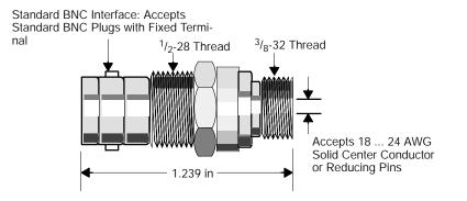
The 52-0370-000 Self-terminating BNC Adapter has a return loss of 40 dB, a frequency range from 100 kHz ... 30 MHz, and an insertion loss of 0.03 dB.
