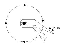
Step 3 f the cable is not fully stripped, squeeze the jaws of the tool together with your thumb and forefinger. Using slight pressure, make one or two revolutions around the cable to cut through the cable jacket.
