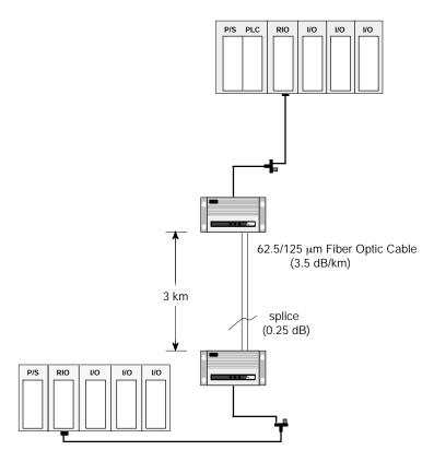
The specified power loss budget for a link using this optical cable is 11 dB. We know that the cable's attenuation over 3 km is 3.5 dB/km x 3 = 10.5 dB, and we are given an attenuation of 0.25 dB for the cable splice. Thus, we have a total optical power loss of 10.75 dB on the link, which is under budget and therefore legal.
