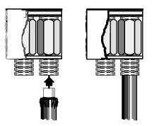
Step 2 Remove the F connector by sliding it out the side of the cassette.
