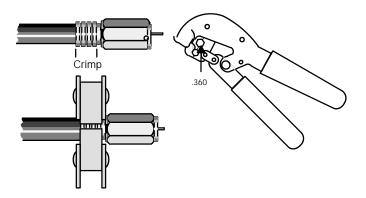
**Step 5** Pull on the F connector to make sure that the crimp is snug—the connector should not fall off.
