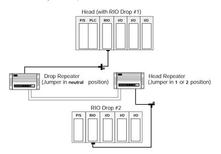
In an optical bus connection, one repeater is always the drop and all other repeaters are heads:
