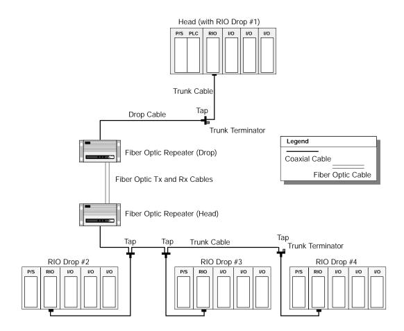
The distance between the two repeaters is limited by the maximum allowable attenuation of the fiber optic cable used in the installation. Fiber attenuation is calculated separately from coaxial cable attenuation (see Section 2.14 on page 43 for details).
