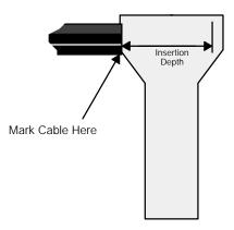
Step 5 Open the jaws and remove the cable. Twist off the cable dielectric and jacket by hand. Remove any long braid strands remaining around the prepared cable end. Long braid strands may be an indication that a new blade pack is needed. Remove any dielectric on the exposed center conductor.
